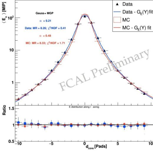
Figure 4: The transverse shower profile  $\langle E_m \rangle$ , as a function of  $d_{core}$  in units of pads, from beam-test data and the MC simulation, after symmetry corrections and fit. The lower part of the figure shows the ratio of the distributions to the fitted function, for the data (blue) and the MC (red).
