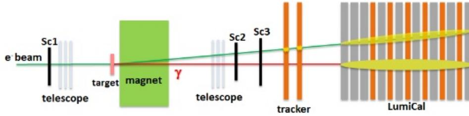
Figure 1: *Test-beam setup, simplified view (not to scale).*
