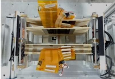
Figure 2: *Top view on the assembled Lumi-Cal prototype*
