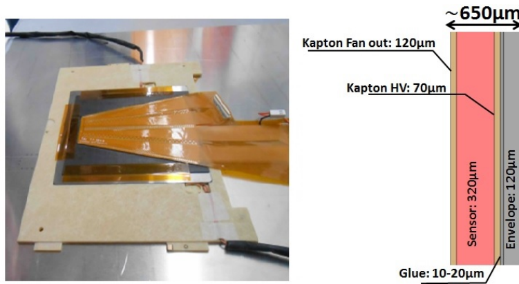
Figure 2: Thin LumiCal module assembly, photo and cross section (not to scale).
